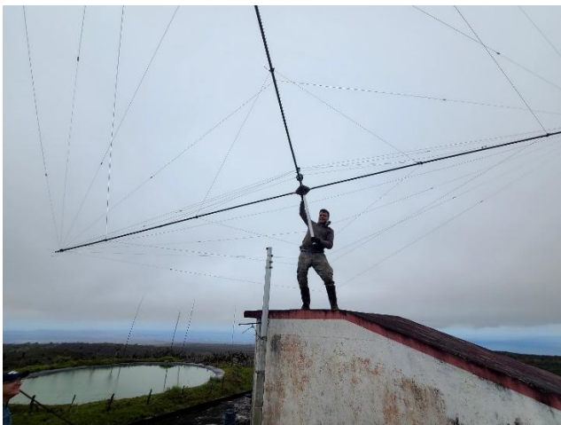
Photo 4 – Manu, LU9ESD, holding the HD8R Spiderbeam that was relocated to the top of the building terrace.
