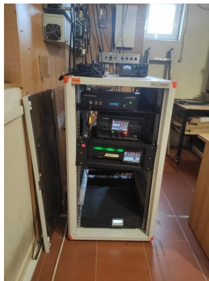
Photo 25 – 4O3A utilizes a FlexRadio 6700 as well as a Power Genius XL amplifier and Tuner Genius XL antenna tuner..
