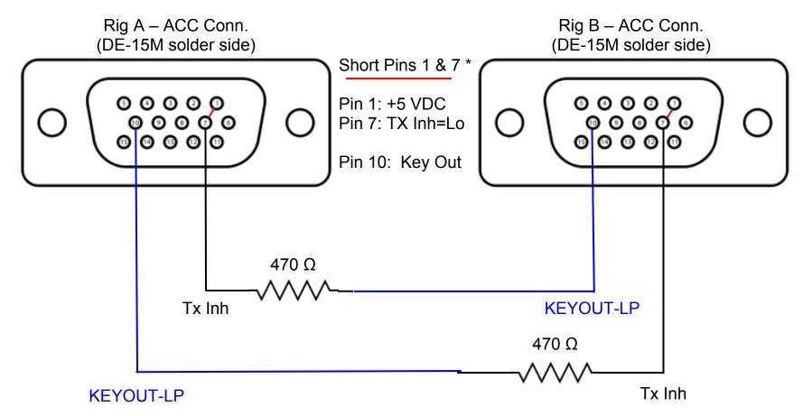
Note: This circuit prevents simultaneous transmission from two K3s, but if both rigs attempt to transmit, <u>neither</u> will transmit (as of K3 Firmware Rev. 4.42).
